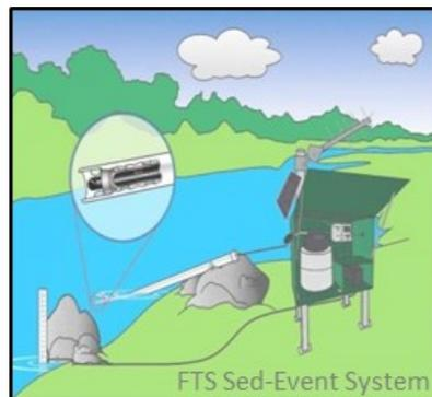
Continuously recorded sensor data, combined with non-continuous water quality analysis, can yield statistical relationships between sensor measurements and constituents that cannot be measured directly. For example, electronic turbidity can be used as a surrogate to accurately calculate suspended sediment concentration (Lewis 1996).
