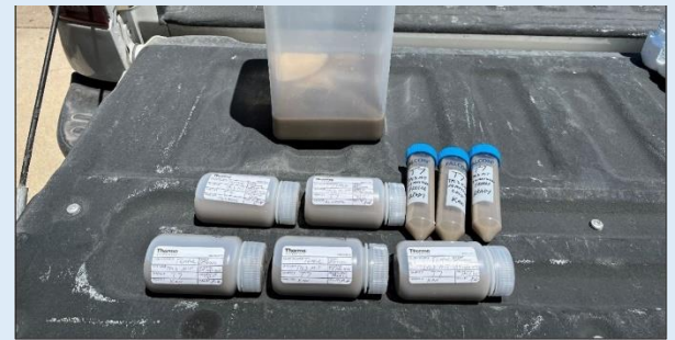
Soil composite sample sub-sampled for shipping to individual labs for analysis.
