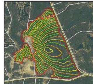
A fire-spread map from BRASS-G. Lines represent 30-min increments.
